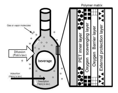
**Figure 1.** Scheme for the general mechanism of gas permeation through a multilayer beverage packaging system including an oxygen scavenger.
