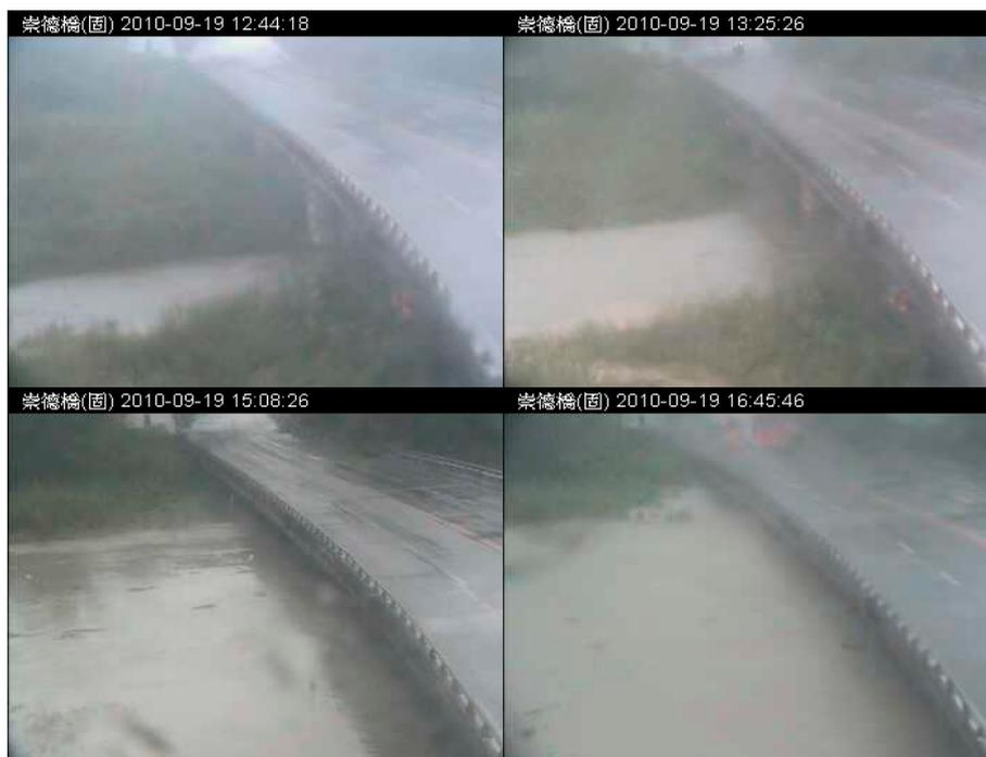
**Figure 4.** Video screenshots from the water-level detection test. This figure has four best-quality images showing representative overflow changes. From top-left to bottom-right, the acquisition time of the four images is 12:44, 13:25, 15:08, and 16:45, respectively. The content of the experiment is the real video of Typhoon Fanapi taken on 19 September 2010, from 12:00 to 18:00 in the afternoon. The experimental images were captured every 1 min during this period, with a total of 350 images.
