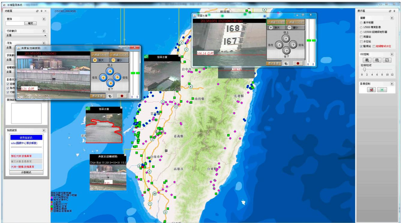
**Figure 6.** Online user interface. Appearance of the hydrological monitoring and flood risk warning system in operation. If any monitoring station reaches a risk level of 80%, the video from the on-site camera directly pops up on the interface, with a red outline indicating the near real-time detected flooding area.
