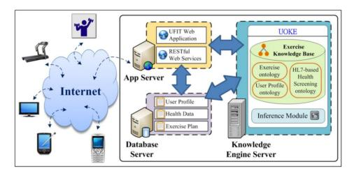
Figure 7. UFIT physical architecture.
