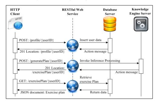
Figure 10. The usage example of REST Service.
