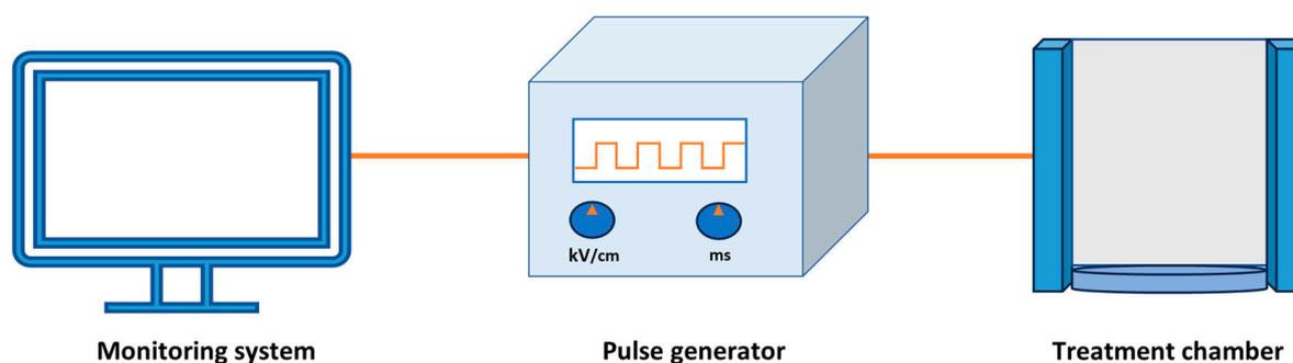
**Figure 1.** A typical PEF apparatus.
