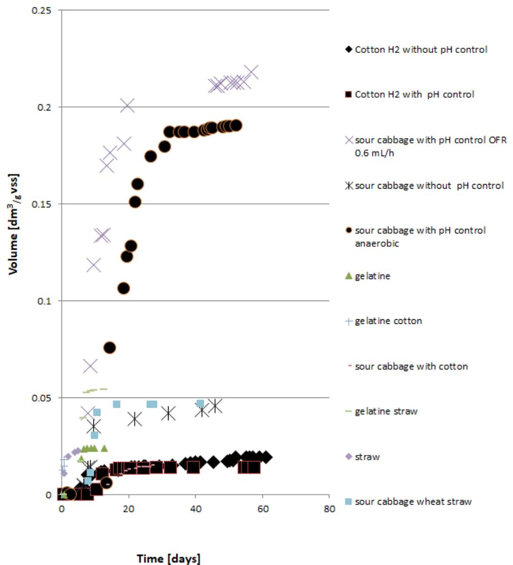
**Figure 2.** Comparison of different substrates' hydrogen yield production for a feed of 20 g VSS/L and compared with data from [51].
