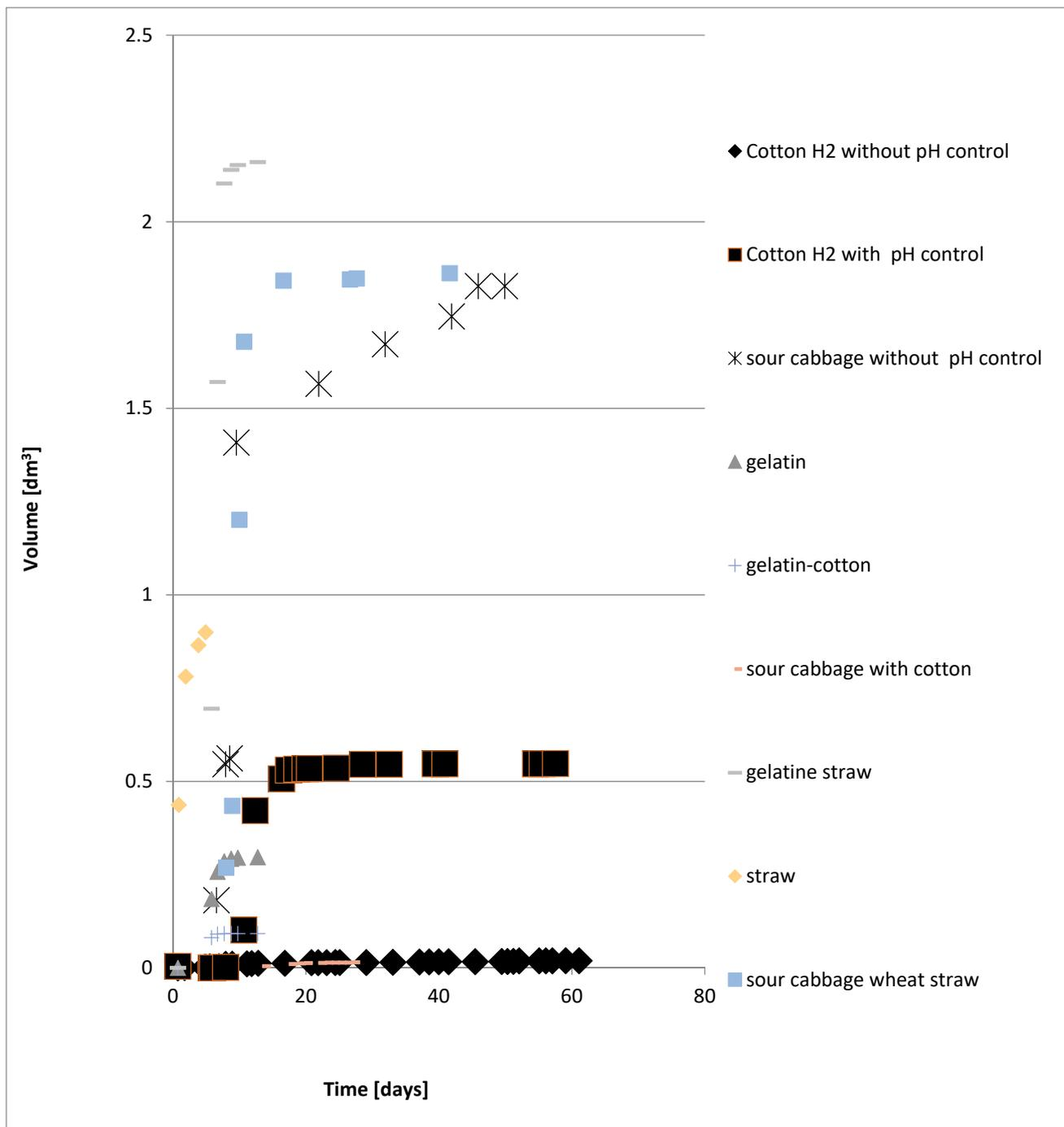
**Figure 3.** Hydrogen sulfide cumulative emission yield from selected feeds.
