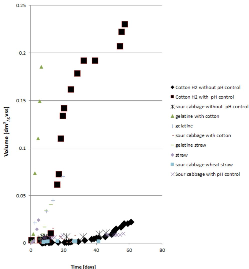
**Figure 5.** Methane production yield from different substrates.
