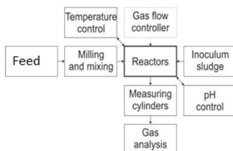
**Figure 1.** Sketch of the experimental procedure for biogas production by dark fermentation of sour cabbage [44] (reproduced with permission from Sołowski Heliyon Elsevier 2021).
