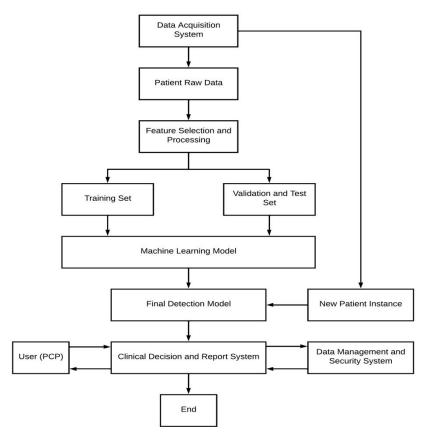
Figure 1. Implementation block diagram for the rheumatic disorder detection system.
