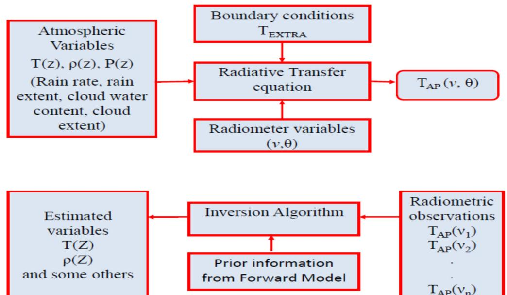
**Figure 1.** Schematic representation of a forward model (**top panel**) used to calculate the brightness temperatures at the different frequencies from the atmospheric variables measured by the radiosonde, where the GMWR measured brightness temperature are not available, and the inverse model (**bottom panel**) used to calculate the atmospheric variables from the estimated brightness temperature. See Rambabu et al. (2013) for more details on a forward model [21].
