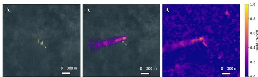
**Figure 2.** Methane emission from offshore O&G platform in Malaysia detected by PRISMA on 24 April 2023. Visualization of O&G platform using Sentinel-2 image (left), methane plume with background Sentinel-2 image (center) and methane retrieval using matched-filter (right).
