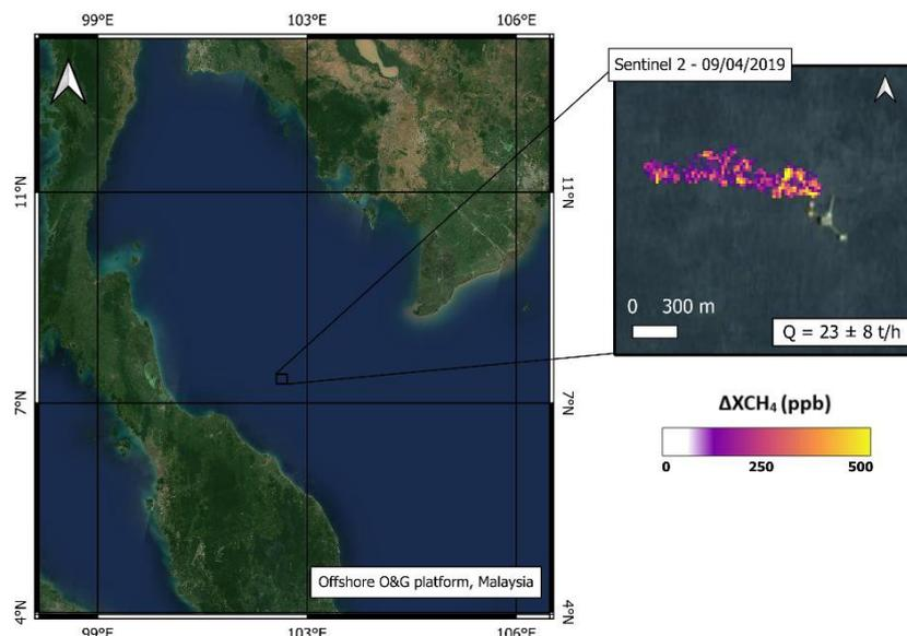
**Figure 1.** The right panel shows a methane emission from offshore O&G platform detected by Sentinel-2 satellite on 9 April 2019. The map on the left panel indicates the location of the platform in Malaysia.
