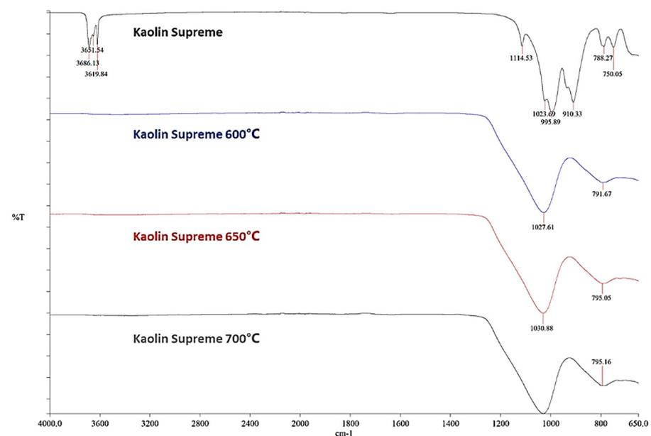
Figure 8. FTIR spectra of Kaolin Supreme and its calcined products at 600, 650 and 700 °C.
