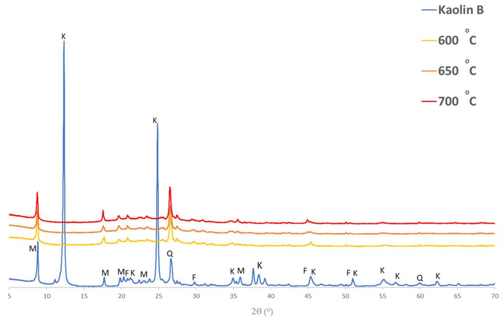
**Figure 2.** XRD patterns for Kaolin B and its calcined products in 600, 650 and 700 °C (K: Kaolinite M: Mica minerals F: Feldspar minerals Q: Quartz).
