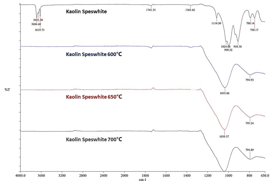
Figure 7. FTIR spectra of Kaolin Speswhite and its calcined products at 600, 650 and 700 °C.
