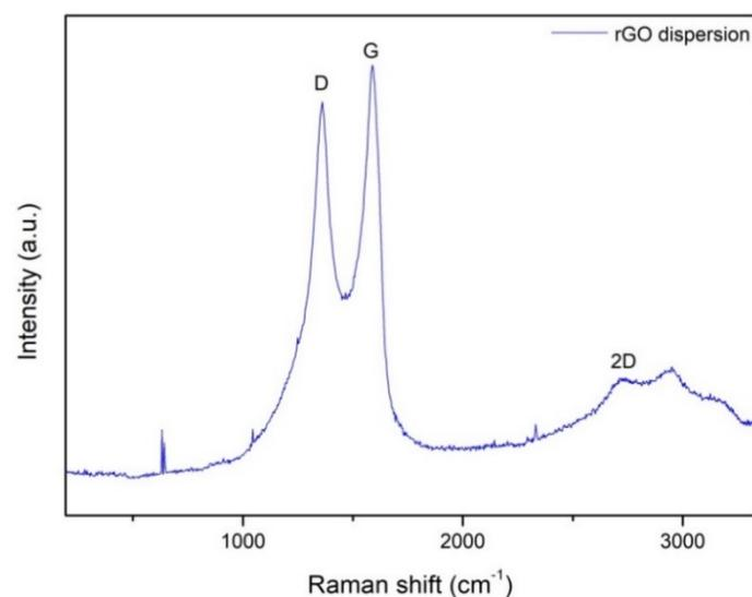
**Figure 2.** Raman spectra of reduced graphene oxide (rGO) dispersion.
