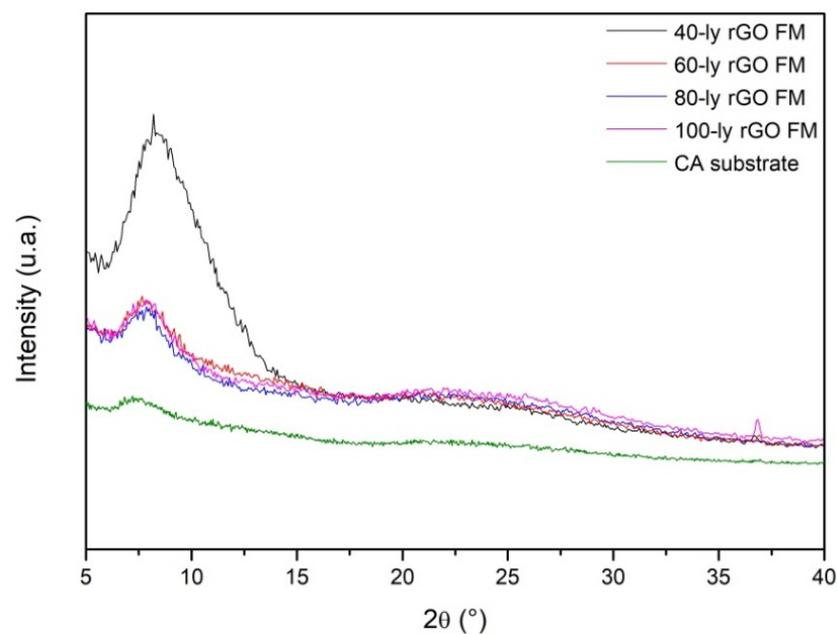
**Figure 4.** XRD patterns for cellulose acetate (CA) substrate and rGO filtration membranes (FM) with different number of layers (ly).
