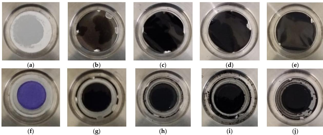
**Figure 7.** Filtration membranes: (a) CA substrate; (b) 40-ly rGO FM; (c) 60-ly rGO FM; (d) 80-ly rGO FM; (e) 100-ly rGO FM before permeation test; (f) CA substrate; (g) 40-ly rGO FM; (h) 60-ly rGO FM; (i) 80-ly rGO FM; (j) 100-ly rGO FM after permeation test.
