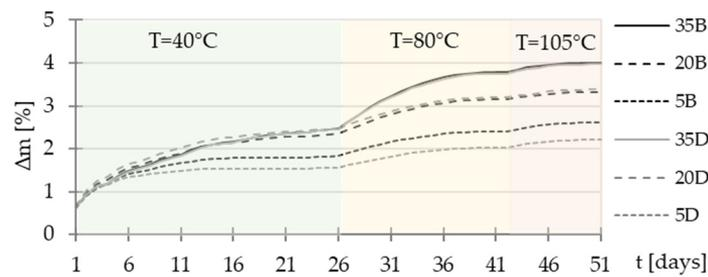
Figure 2. Scheme of drying process.
