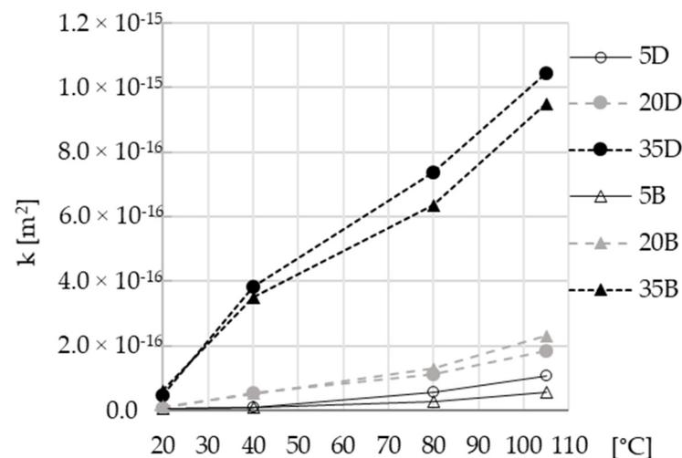
**Figure 4.** Impact of drying temperature on gas permeability of AAC.
