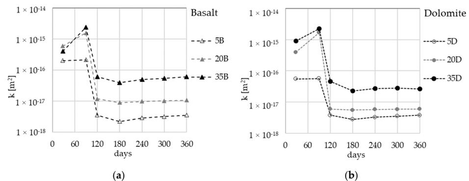
**Figure 1.** Gas permeability development in time for samples stored in room conditions: (a) basalt aggregate; (b) dolomite aggregate.
