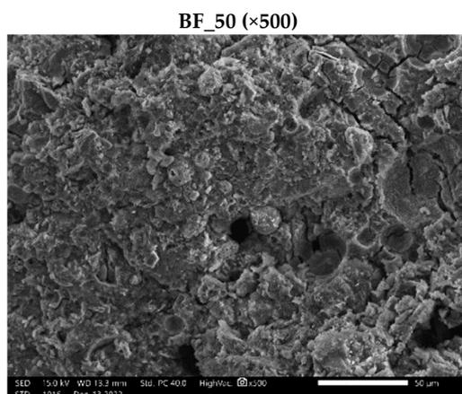
**Figure 7.** The microstructure SEM photography of produced geopolymers.
