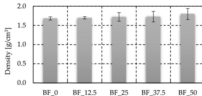
**Figure 4.** The density of the tested geopolymers.
