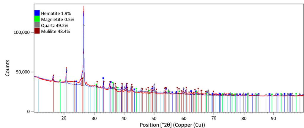
Figure 2. Diffractogram for fly ash.
