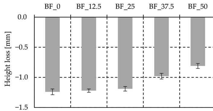
**Figure 6.** The height loss of tested geopolymers due to abrasion test.
