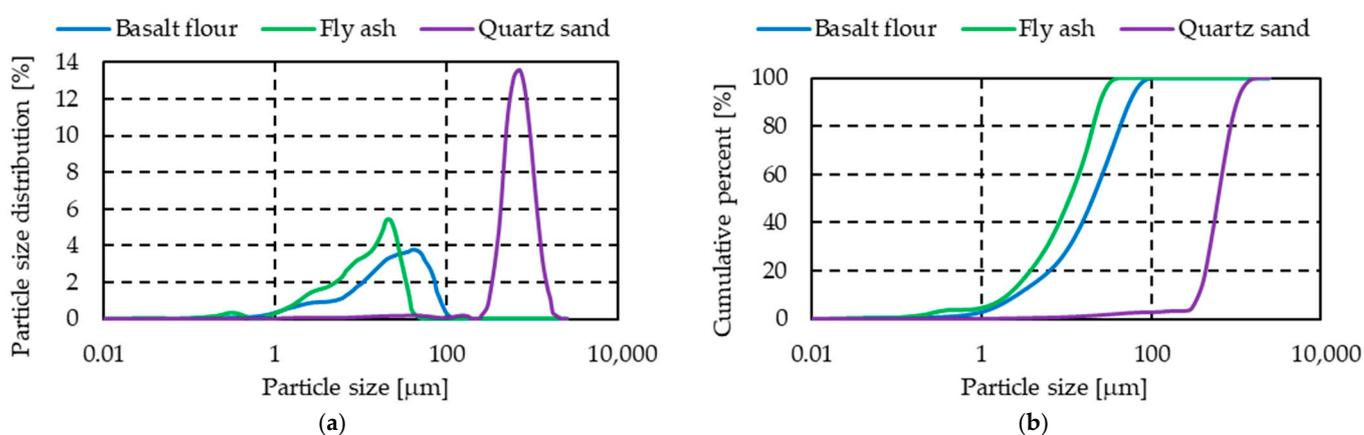
**Figure 3.** (a) The particle size distribution curves for fly ash, quartz sand, and basalt flour; (b) the cumulative curves for fly ash, quartz sand, and basalt flour.
