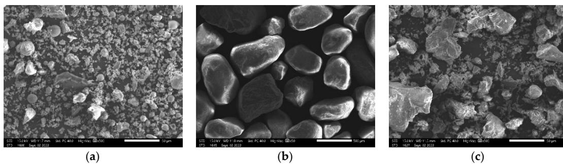
Figure 1. SEM micrographs of (a) fly ash, (b) quartz sand, (c) basalt flour.
