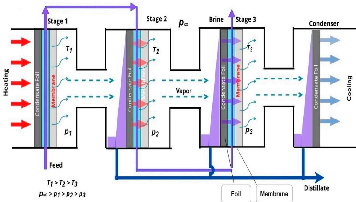
Figure 1. Schematic diagram of MD unit showing evaporation–condensation stages.
