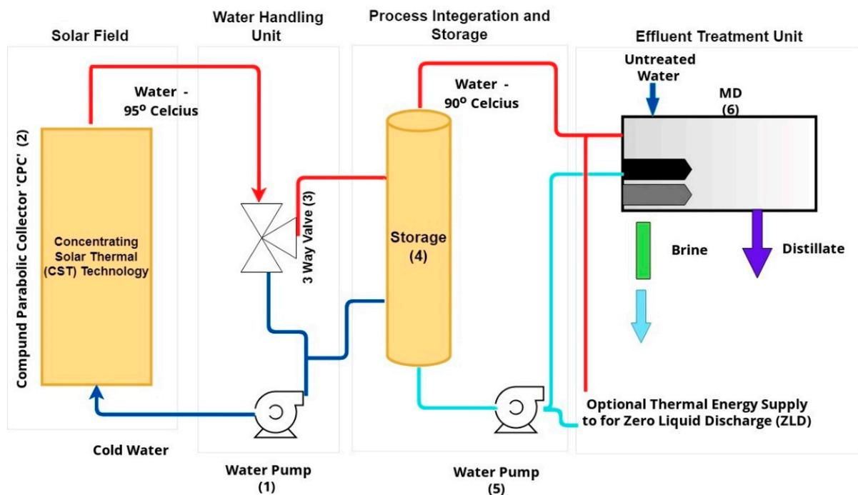
**Figure 2.** A schematic representation of the design of solar-based waste treatment system at the experimental textile unit.
