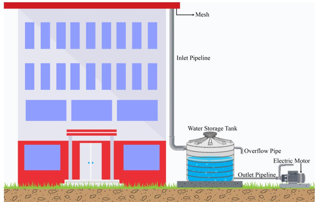
**Figure 3.** Schematic diagram of a rooftop harvesting system.
