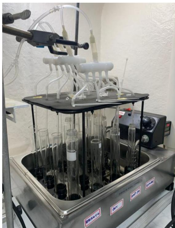
**Figure 3.** Bench-top accelerated oxidation system used in the proposed method to assess the oxidative stability of the safflower and babassu biodiesels.
