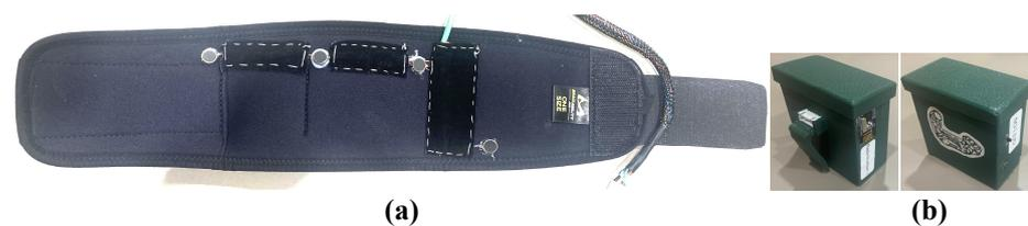
**Figure 14.** (a) Manufactured sensory feedback armband, (b) electronics box.
