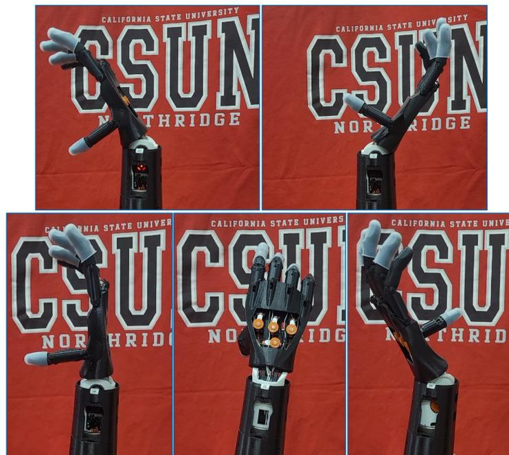
**Figure 23.** Wrist bending and rotation.
