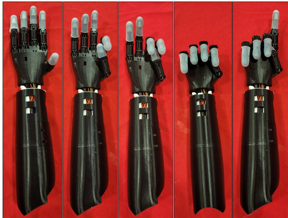
**Figure 20.** Five grip patterns (relax, pinch, tripod, power, and point).
