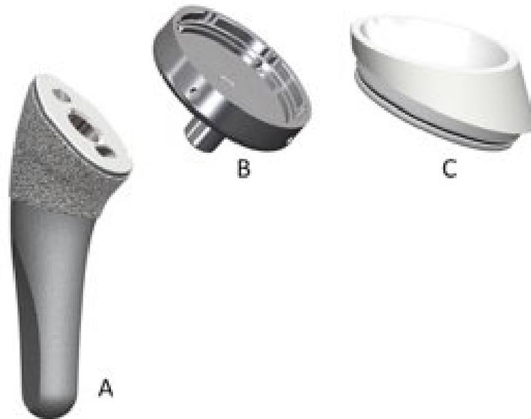
**Figure 5.** Short-stem lateralized humeral component of reverse shoulder arthroplasty. (A) A hydroxyapatite-coated curved short-stem 132.5° inclination; (B) an eccentric (+1.5 mm and +3.5 mm) reverse tray; and (C) an asymmetric polyethylene insert (thickness + 6 mm and + 9 mm) with 12.5° inclination (Stryker, Kalamazoo, MI, USA).
