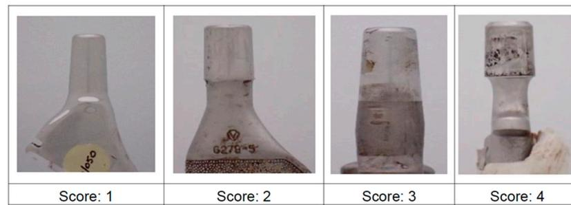
**Figure 1.** An example of the fretting corrosion damage scoring of the trunnion [29].
