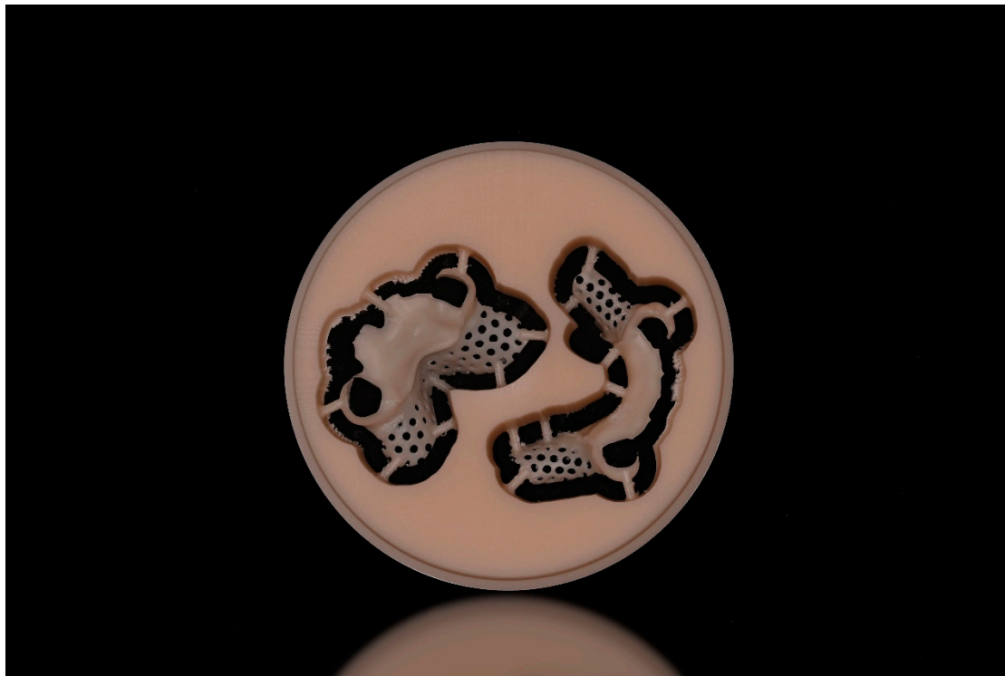
Figure 2. Milled polymer-based frameworks with supports in place. After removal of the supports, frameworks require finishing and polishing prior to beginning tooth setting.
