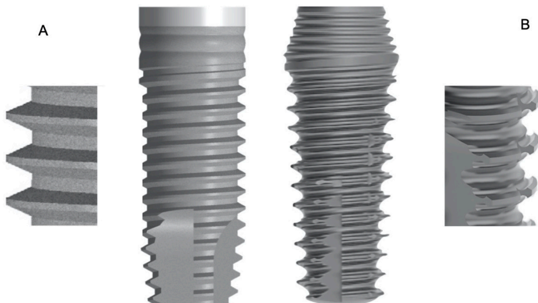
Figure 1. (A) control cylindric implant with “V” thread; (B) test new tapered implant with reverse conical collar and “nest shape” thread.
