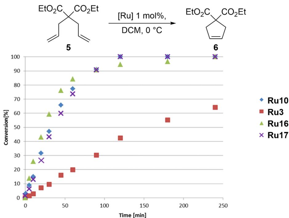
**Figure 5.** Relative conversion rates for a model RCM reaction of **5** using 1 mol% of the catalyst.
