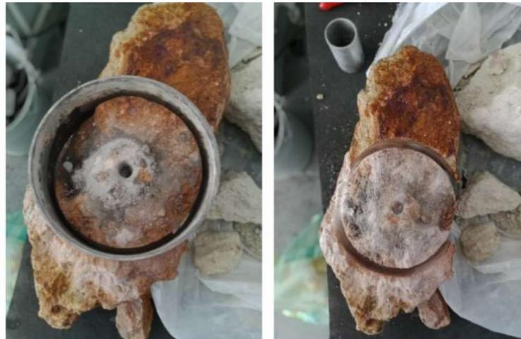
**Figure 6.** Rock sample from Hallaç Complex, which could not be cut to be used for impedance tube testing.
