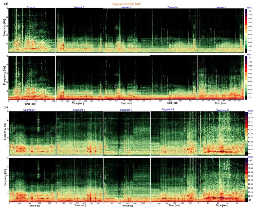
**Figure 6.** The spectrograms for all five segments for Taoyuan International Airport MRT while traveling from (a) Airport Terminal II to Taipei station and (b) Taipei station to Airport Terminal II. The spectrograms are presented in dB(A) and dB(C) scales.
