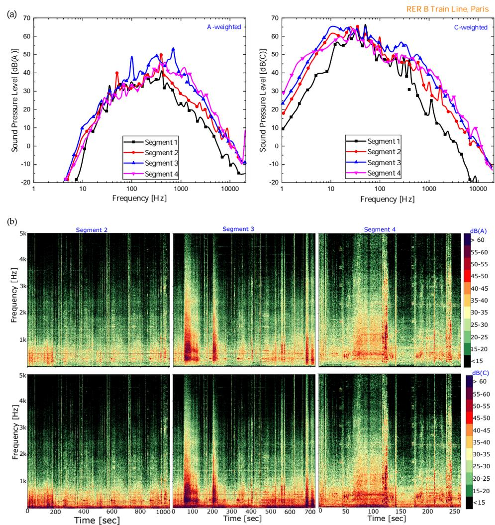
**Figure 9.** (a) Sound pressure level spectrum of four segments measured for RER B Paris while traveling from Gare du Nord to CDG airport. (b) The corresponding spectrograms for segment 2 (left), 3 (middle), and 4 (right) for RER B train line Paris in dB(A) and dB(C) scales.
