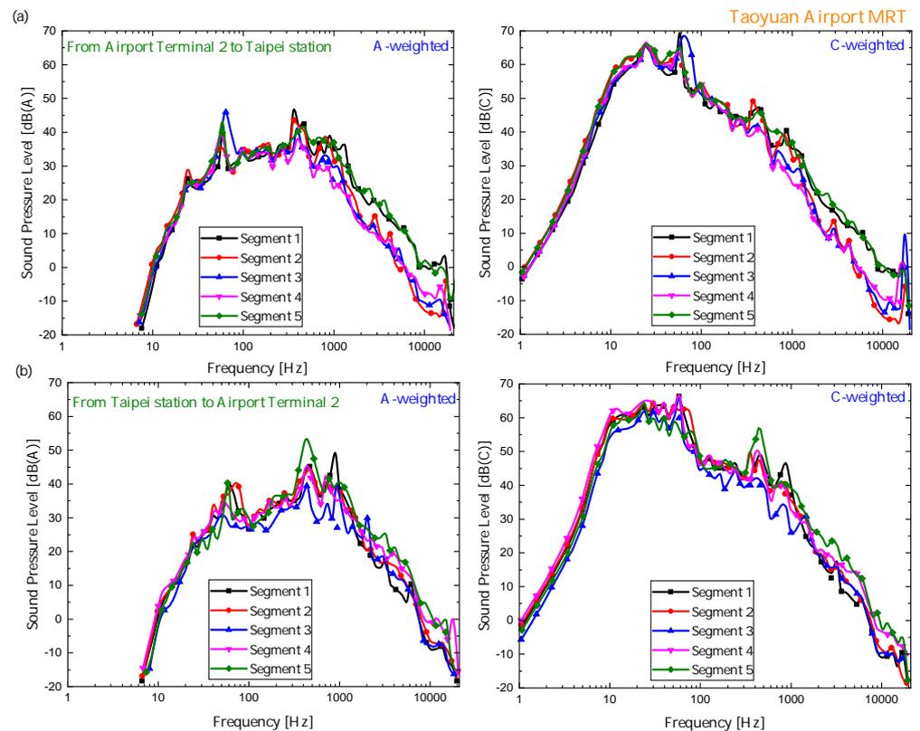
**Figure 5.** Sound pressure level spectrum of the five segments measured for Taoyuan Airport MRT while (a) Travelling from Airport Terminal 2 to Taipei station, and (b) Travelling from Taipei station to Airport Terminal 2.
