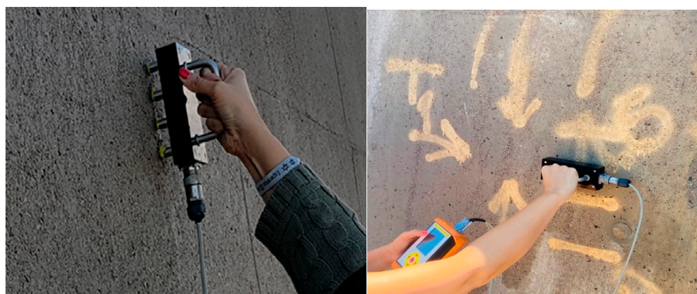
Figure 8. Electrical resistivity measurements with a Wenner probe equipment.
