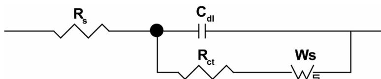
**Figure S4.** Equivalent circuit for the Nyquist plots of the EIS measured for the SAM of **2** on Si–H and the fresh Si–H surfaces.  $R_{ct}$  of  $\sim 1187$  Ω and  $\sim 4571$  Ω for the bare Si–H and the functionalized Si surface respectively, is expected on the basis that a monolayer can partially block charge transfer at the interface and therefore increase the charge transfer resistance.
