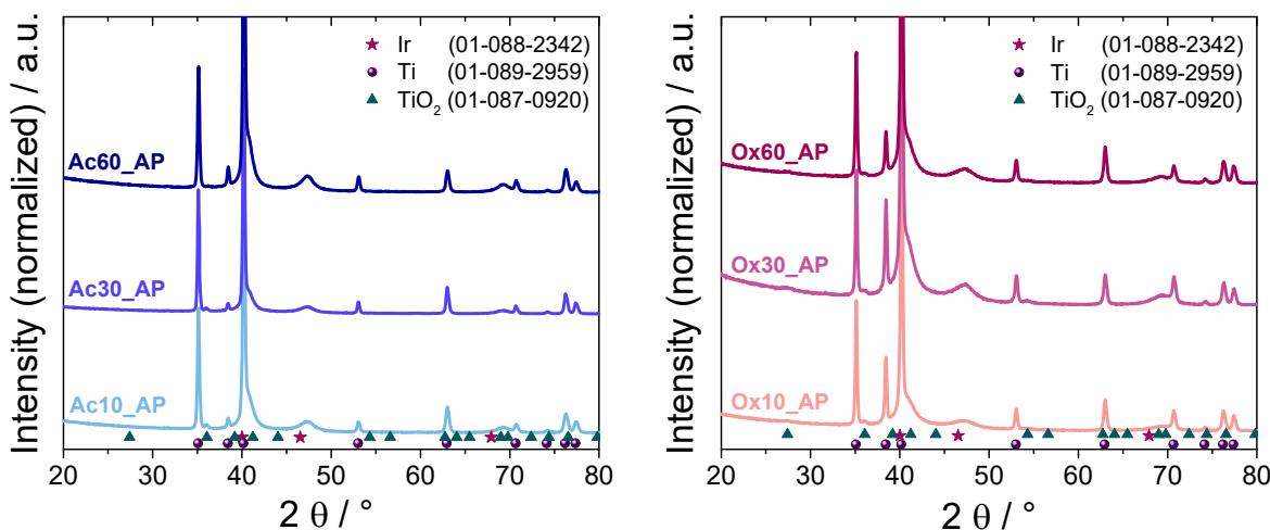
**Figure S2.** X-ray diffraction (XRD) of the as-prepared Ac and Ox films (\_AP) show no major changes in the crystal structure in dependence of heating time. The large reflections can be attributed to the rutile phase of Ti.
