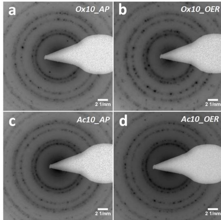
**Figure S4.** Selected area diffraction (SAED) images of the scraped \_AP and \_OER films of (a) Ox10\_AP, (b) Ox10\_OER, (c) Ac10\_AP and (d) Ac10\_OER.
