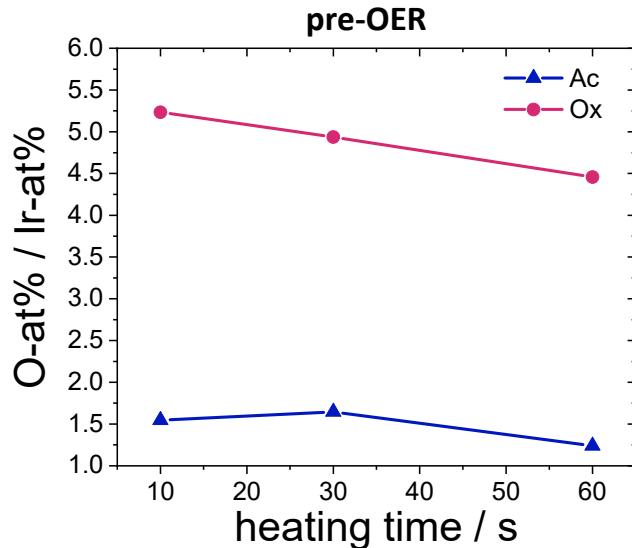
**Figure S1.** EDX results of \_AP Ox and Ac films showing the atomic percentage (at%) ratio of O to Ir measured with 6 keV. Independent of heating time the Ox films exhibit a significant higher oxygen amount than the Ac films.
