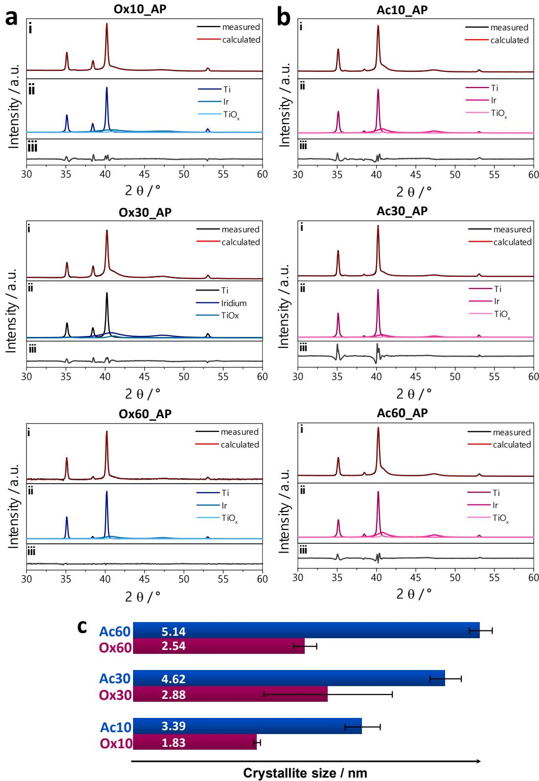
**Figure S3.** Grazing incidence X-ray diffraction measurement of \_AP Ox (a) and Ac (b) samples on Ti substrate with (i) measured and calculated diffraction pattern from Rietveld refinement results. (ii) The Ti, Ir and  $\text{TiO}_x$  phases, which were used within the refinement. (iii) The difference between measured and calculated diffraction pattern. (c) Crystallite sizes of \_AP samples obtained by quantitative Rietveld analysis are given in white in the respective bar.
