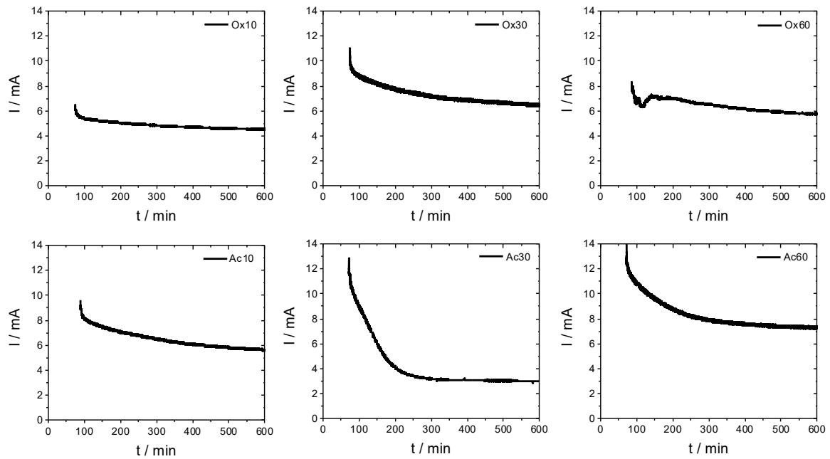
**Figure S8.** Stability measurements of Ox and Ac films in 0.05 M  $\text{H}_2\text{SO}_4$  at 1.734 V<sub>RHE</sub> (not IR corrected). The catalysts show a major loss of current in the beginning before running in to an almost stationary plateau, an approach to steady-state after quick potential change.
