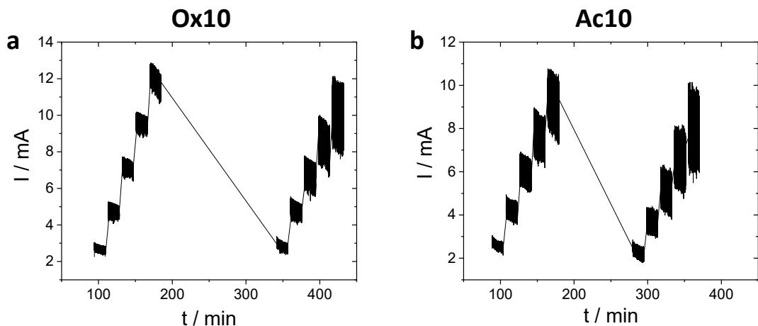
**Figure S7.** Stepped potential voltammetries (SPVs) exemplarily shown for Ox10 and Ac10. The non-stationary behavior of the potential steps may be caused by instabilities of the catalyst.
