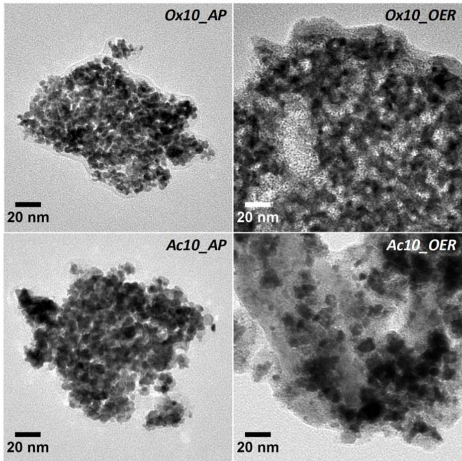
**Figure S6.** TEM images of the scraped \_AP and \_OER films displaying crystalline Ir particles.
