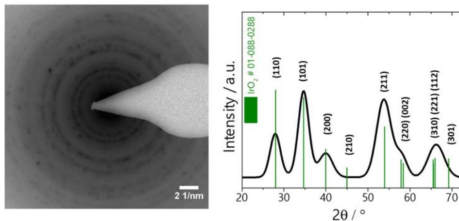
**Figure S5.** SAED and evaluated diffraction pattern of an  $\text{IrO}_x$  film reveals a rutile-type phase.
