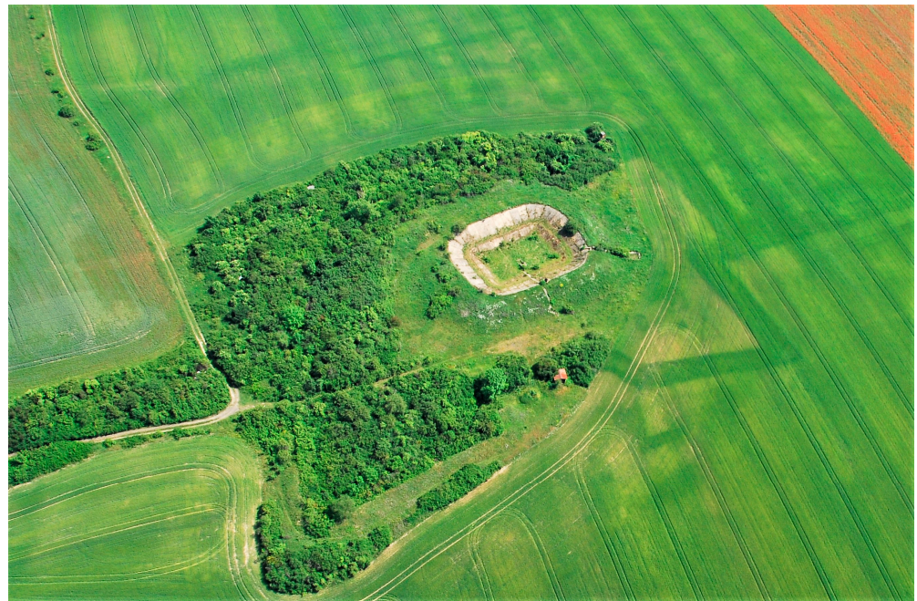
Figure 5. Semi-ruined earthworks of an artillery fort, part of the Třeboutice linear defensive system constructed near the district town Litoměřice. Part of its former rectilinear perimeter ditch (the dark-green zig-zag line) is now filled in and is visible through cropmarks produced by barley growing above it) and 7 this fort is marked by white arrows. In the original plan made in 1860 this fort is labeled Werk III.
