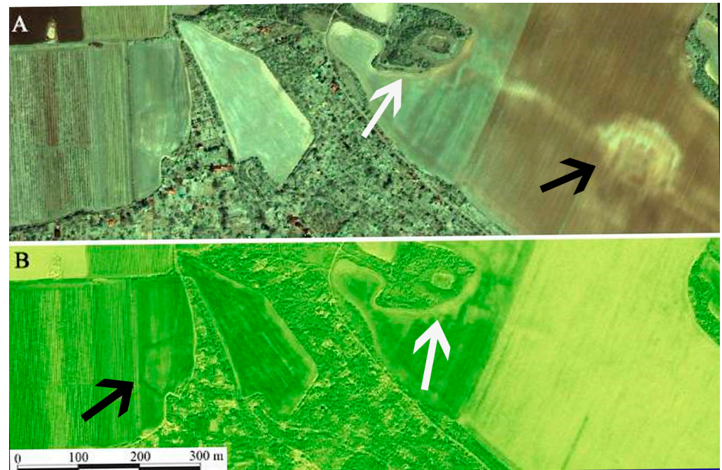
Figure 7. The Třeboutice linear defensive system on satellite images captured by QuickBird-2 on 3rd May 2006. (A) Combination of multispectral images (spatial resolution 0.61 m) in visible spectral band (R + G + B) adapted with pan sharpening; (B) result of the calculation of the normalized ratio vegetation index (NRVI) by the IDRISI software (also pan sharpened). After: [66].
