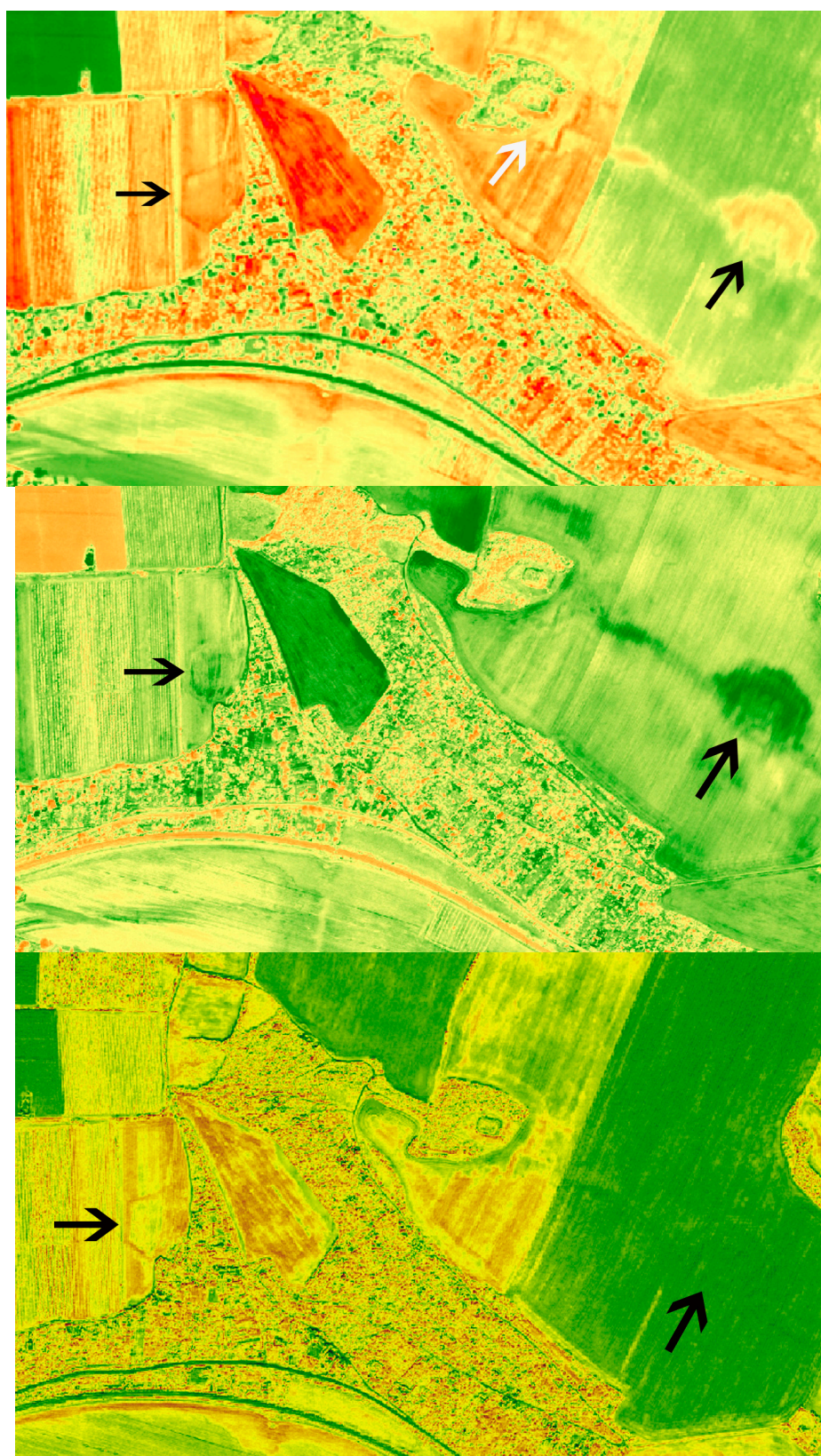
Figure 6. The linear defensive system composed of artillery forts in Třeboutice (district Litoměřice)—one semi-ruined (white arrow) and two completely buried (black arrows), as scanned on 3 May 2006 by QuickBird-2, displayed in the following spectral bands: top —NIR, center —Red, bottom —NRVI. The present author's project, University of West Bohemia.
