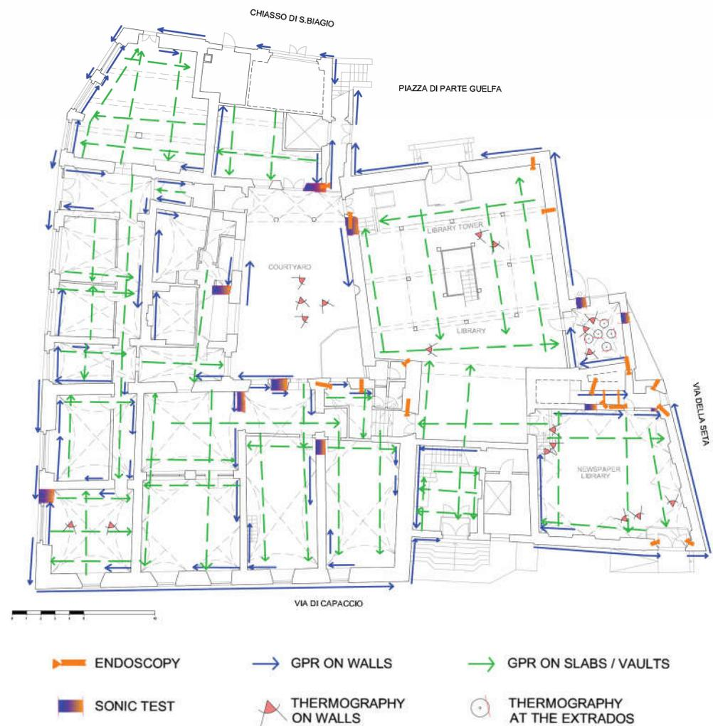
**Figure 7.** The ground floor plan of the building with the investigations carried out. Other layout diagrams are included in Appendix A.
