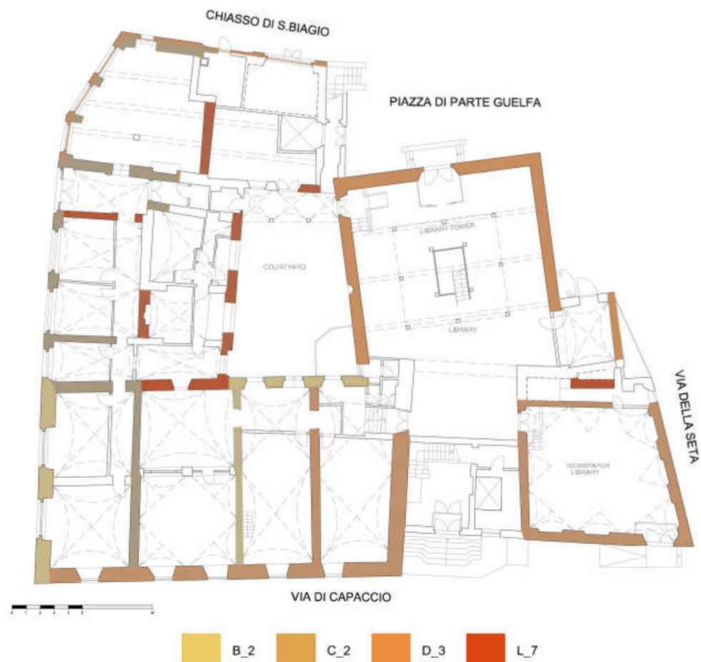
Figure 8. Layout of the building showing the identified typologies.
