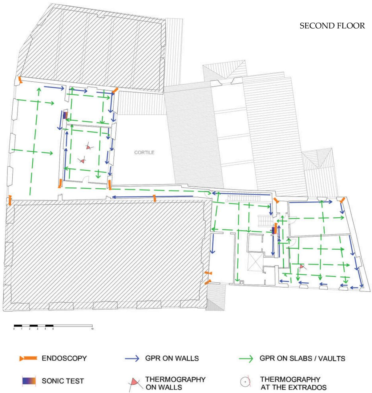
**Figure A1.** Investigations carried out on the different parts of the building.
