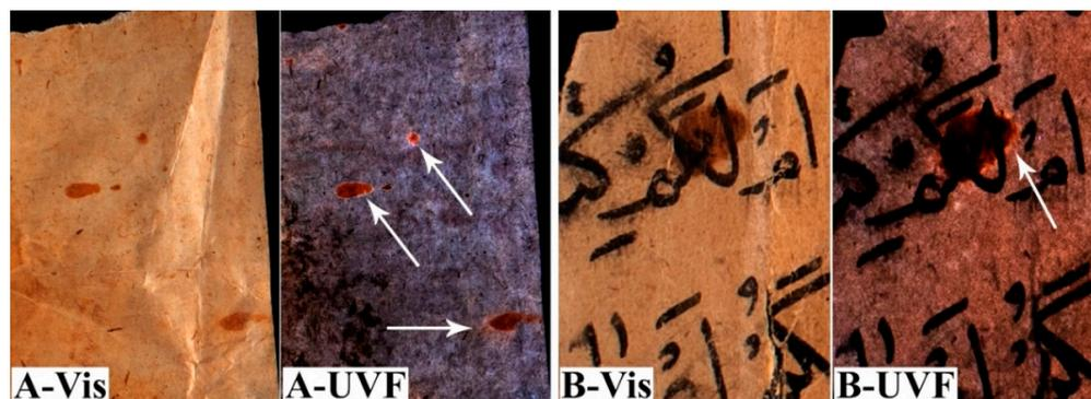
**Figure 3.** Photographic imaging of two foxing spot on two different papers (A and B) of manuscript; Vis: visible reflected light, UVF: Ultraviolet fluorescence.
