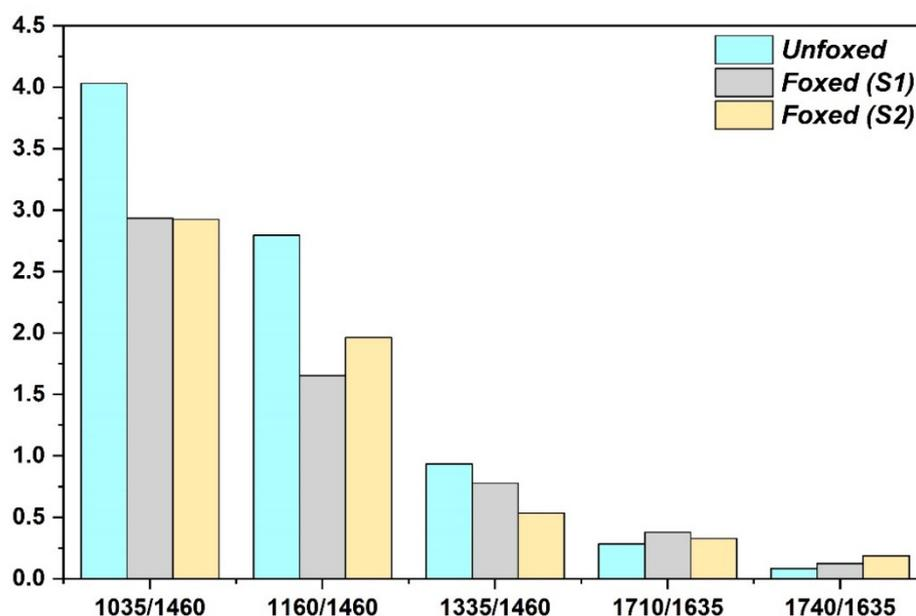
**Figure 6.** Peaks intensity ratios as oxidation indices of cellulose in the FTIR spectra of unfoxed and foxed papers.
