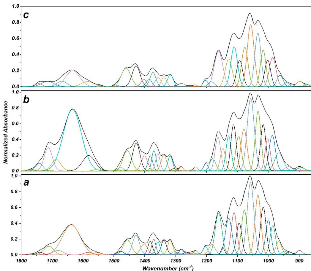
**Figure 5.** Gaussian peak deconvolution of FTIR spectra of foxed (b: S1, c: S2) and unfoxed (a) papers, baseline corrected in the region of 850–1800  $\text{cm}^{-1}$ .
