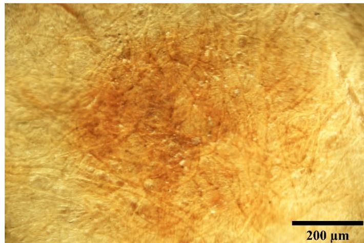
**Figure 7.** Discoloration of paper fibers to yellow-brown in foxing stains as a result of cellulose oxidation.
