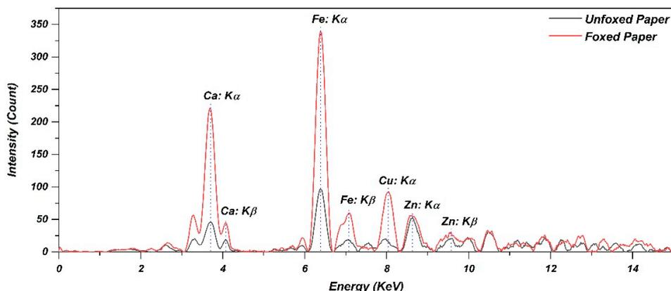
**Figure 4.** XRF spectra of paper with and without foxing stains that show increased levels of iron, copper and calcium in the foxed area.
