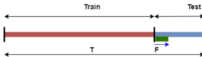
**Figure 5.** Data partitioning for training and prediction experiments.  $T$  is the duration of the dataset (1810 time samples = 905 days),  $F$  the length of the prediction window (14 samples = 7 days), and the blue line is the testing period which includes 20 forecast sliding windows, each separated by a 12 h period.
