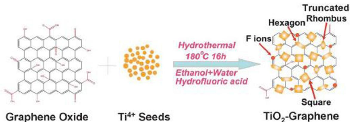
**Figure 14.** Schematics for the preparation of graphene/TiO<sub>2</sub> nanocomposites by a hydrothermal treatment in the solvent of ethanol, water and HF. (Reprinted with the permission of ref. [128], copyrights 2012 © Royal Society of Chemistry.
