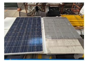
**Figure 1.** The solar panel situated on the left-hand side has reached its end of life, while the solar panel located on the right-hand side has undergone partial delamination.
