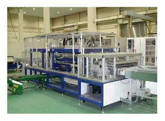
**Figure 6.** Module delamination involves glass and EVA separating equipment (Photo courtesy of NPC Incorporated) [20].
