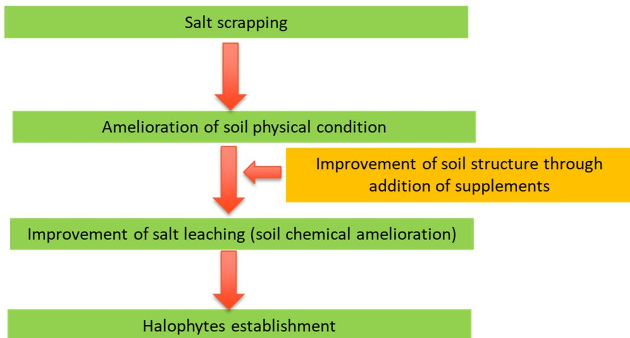
**Figure 1.** The diagram indicating the techniques required for reclamation of salt-affected land.
