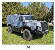
**Figure 4.** Autonomous vehicle type RDO 3927 KOMONDOR with a rescue (**a**) and reconnaissance (**b**) superstructure. Source: author's picture.
