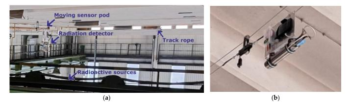
**Figure 9.** (a) Wire ropeway path with a motorised automatic detector moving mechanism. (b) RadNDI scintillation detector attached to the wire ropeway. Source: the author's own source.
