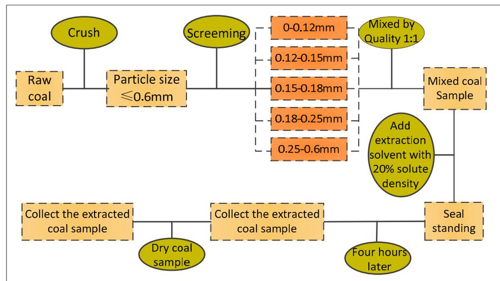
**Figure 4.** Flow chart summarizing the experimental procedure.
