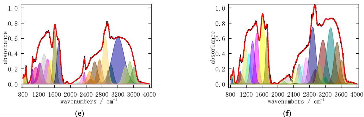
**Figure 7.** Peak fitting results for FTIR spectra acquired from coal samples extracted using (a) MT, (b) CYH, (c) n-hexane, (d) CYH + AOT + AE, (e) AE and (f) AOT.
