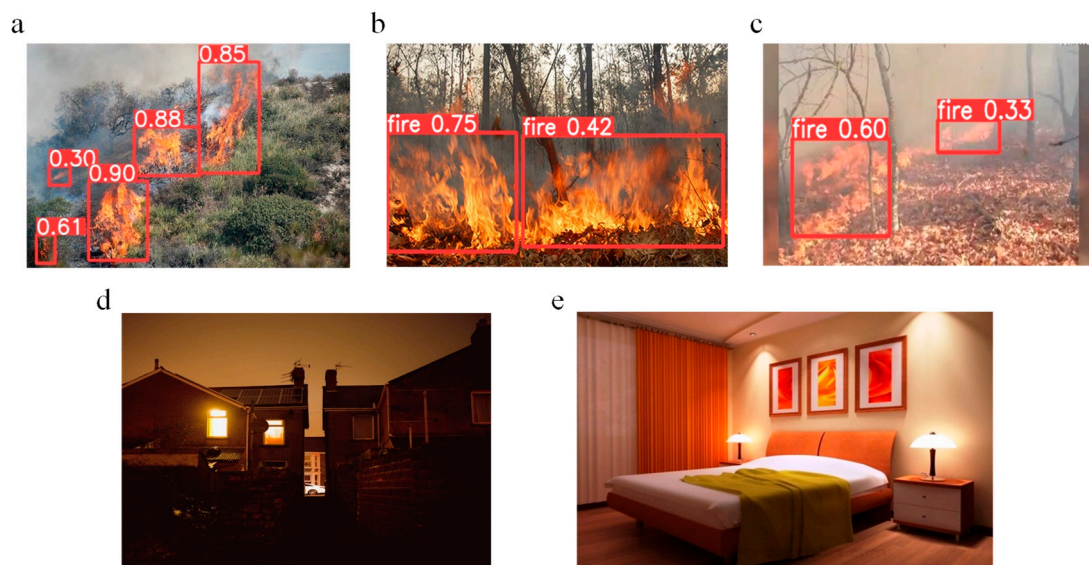
Figure 15. Flame detection with YOLOv5n model based on images from the Internet, including: (a) forest canopy flames, (b,c) woodland ground flames, (d,e) flame-like targets.
