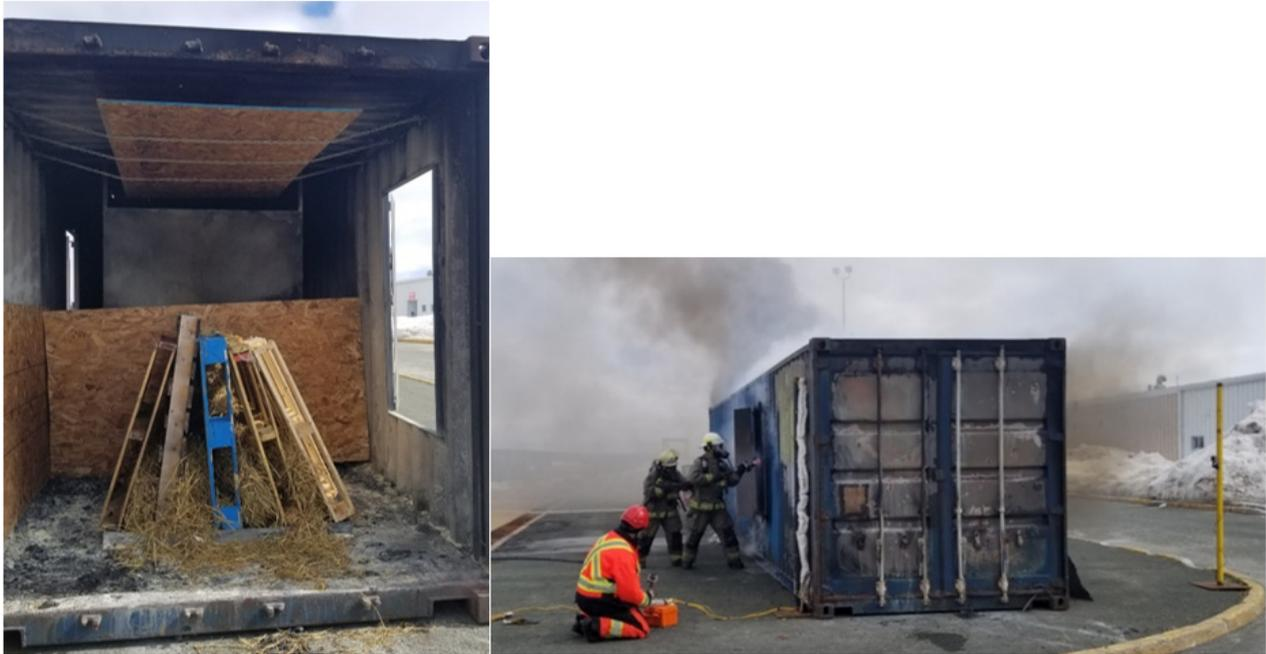
**Figure 2.** Images showing the set-up of the fuel load in the burn room and the location of the GoPro cameras, thermocouple array, and fire fighters during a trial.
