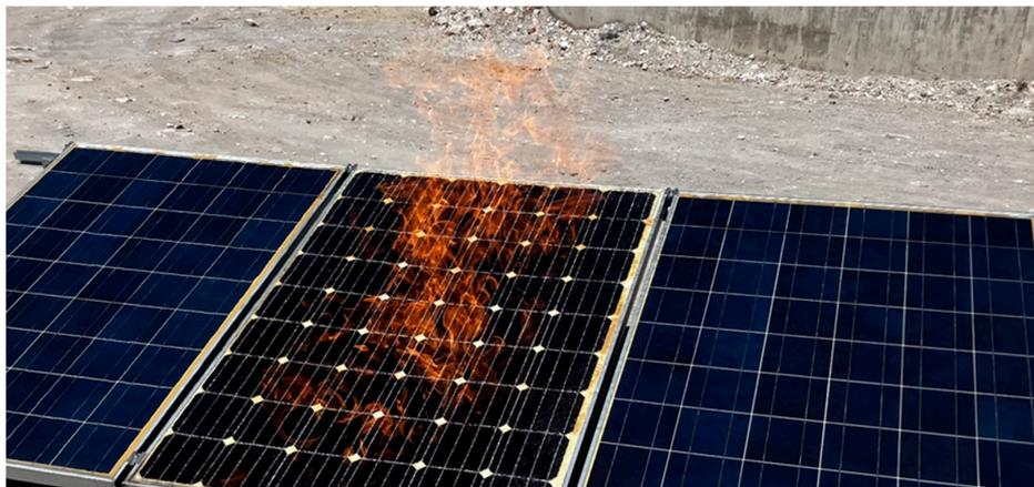
Figure 6. Visualization of a fire caused by a hotspot in a PVM in ENES J-UNAM.
