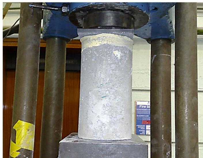
**Figure 4.** Setup for axial compression test to determine the compressive strength of LFC.
