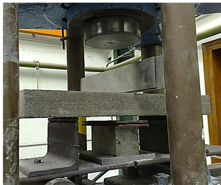
**Figure 5.** Setup for three-point bending test to determine the flexural strength of LFC.
