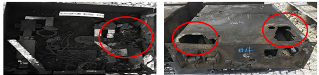
Figure 4. Fires in energy storage system module [25].
