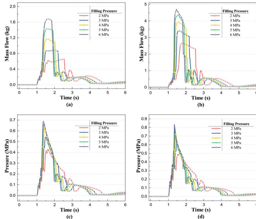
**Figure 5.** Mass flow rate and pressures change at nozzle under different filling pressures: (a) Mass flow in long branch; (b) Mass flow in short branch; (c) Nozzle pressures for long branch pipes; (d) Nozzle pressures for long branch pipes.
