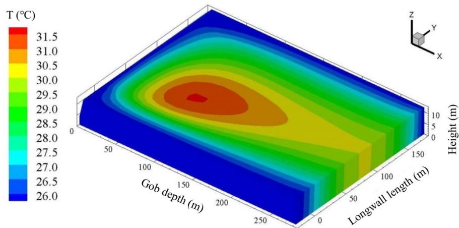
Figure 10. Simulation result of the temperature distribution in the goaf area.
