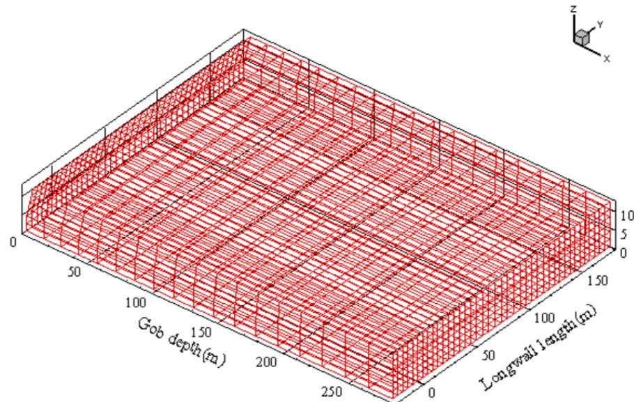
Figure 9. Mesh generation of the model of the goaf area.
