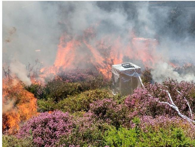
**Figure 2.** Field test (PSS) views during the arrival of the fire front at the protective device of the gas cylinder.
