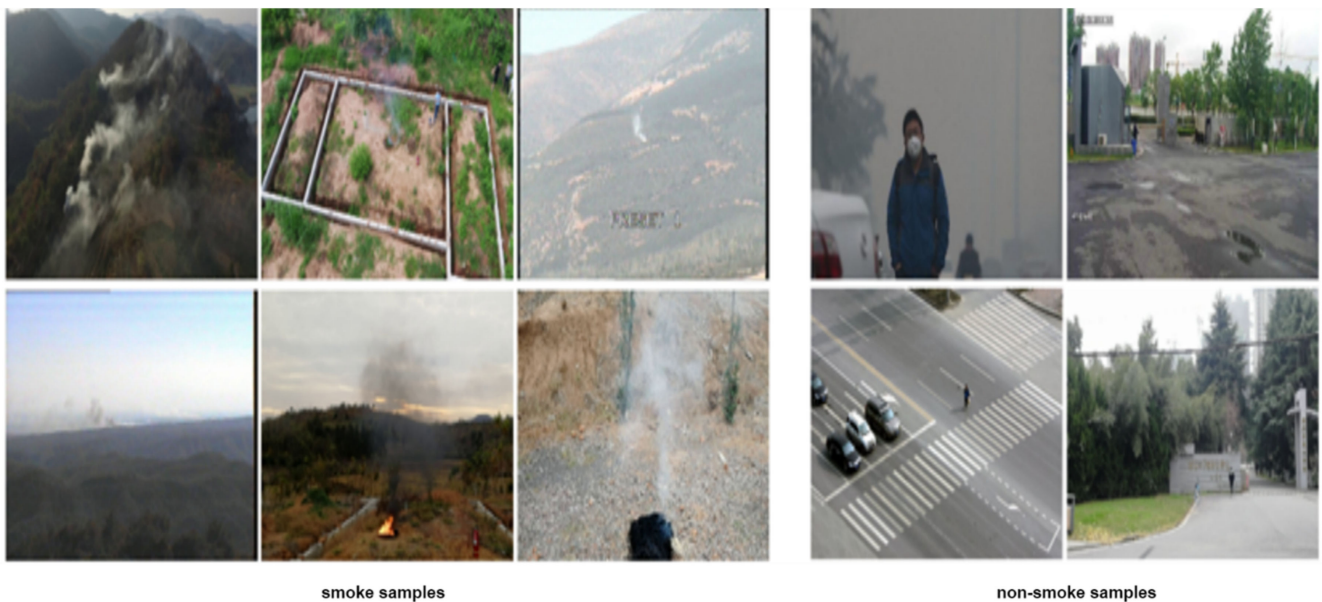
Figure 6. A view of smoke samples. Smoke instances are extra small and of less density with a challenging background. Non-smoke images are also challenging with moving trees, cars, and persons.
