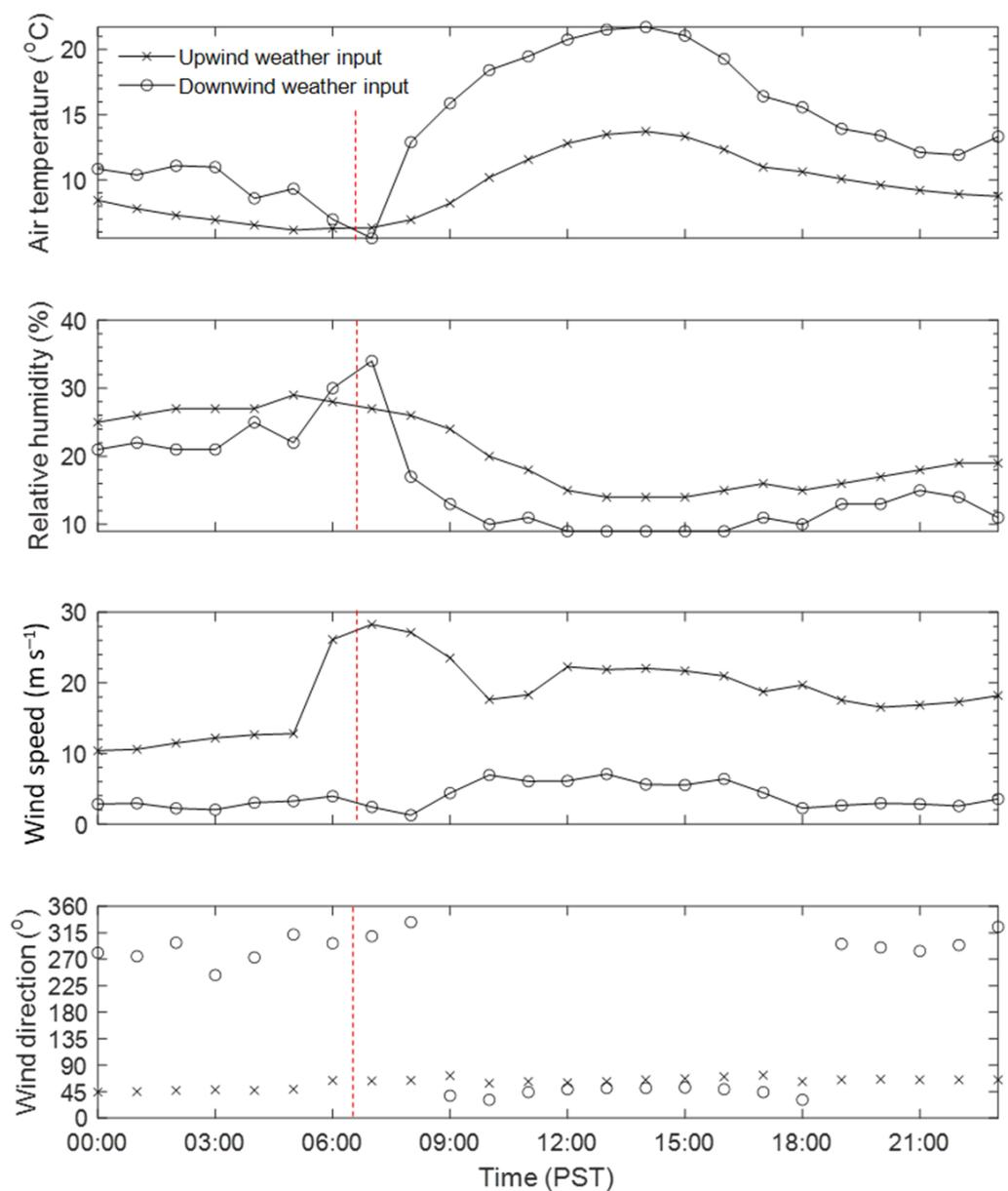
**Figure 2.** Input weather stream used in the Prometheus fire growth model simulations. The dashed red vertical line indicates approximate fire ignition time (06:25 PST). The locations of the upwind and downwind weather stream inputs are shown in Figure 1.
