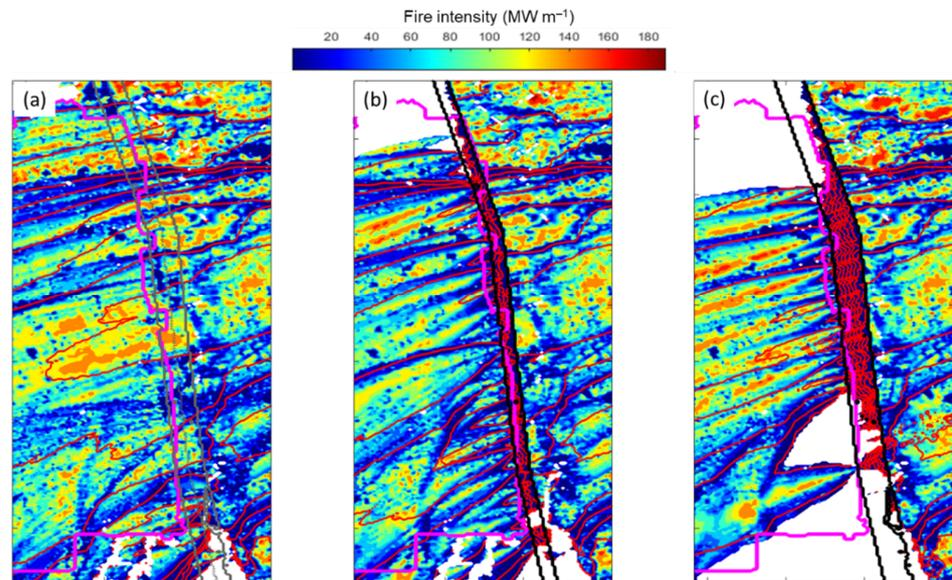
**Figure 5.** Simulated fire intensity of the 2018 Camp Fire for the: (a) no WUI-FB; (b) WUI-FB200; and (c) WUI-FB400 scenarios. Red contours indicate fire propagations and thick magenta lines indicate the Paradise Township boundary. The locations of the WUI fuel break are indicated by a black polygon. The WUI fuel break location shown in (a) is only for reference.
