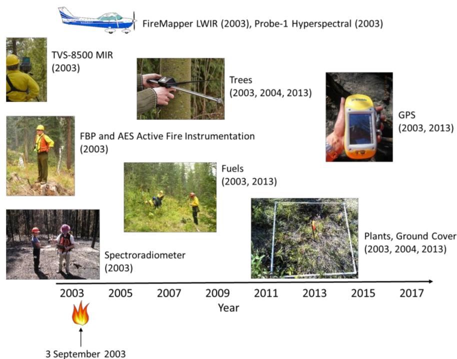
Figure 2. Overview of the different types of pre-fire, active fire, and post-fire datasets collected at the Cooney Ridge Fire Experiment on 3 September 2003, and years of data collection. LWIR: Long-Wave Infrared; MIR: Middle Infrared; GPS: Global Positioning System; FBP: Fire Behavior Package; AES: Autonomous Environmental Sentry.
