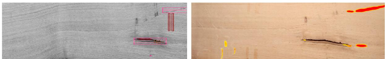
**Figure 10.** Defect detection on specimen 8 (**left**—software 1 image; **right**—software 2 image).
