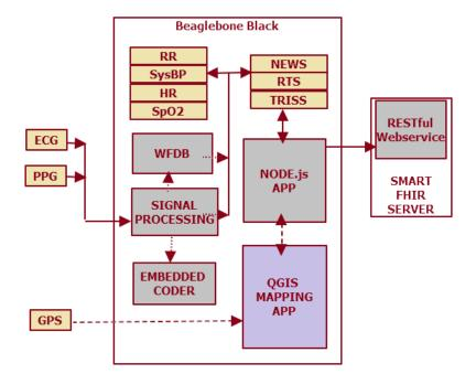
**Figure 1.** Composite sensor kit architecture showing all the data acquisition, signal processing, and computing components
