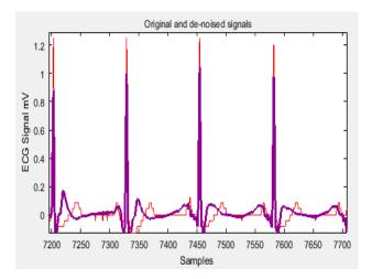
**Figure 4.** Noise removal in the ECG signal using stationary wavelet transforms 1-D (MATLAB) using 'sym4' wavelet and level '5' decomposition. The de-noised, corrected signal shown overlaying the noisy signal. The ECG signal was used to derive the heart rate and arterial blood pressure using Physionet WFDB library.
