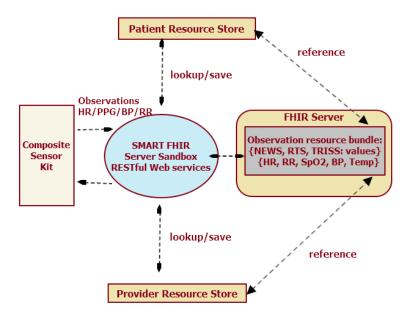
**Figure 3.** SMART FHIR server architecture showing the RESTful Web services that could be accessed from an embedded system hardware (Beaglebone Black).
