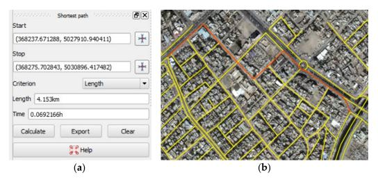
**Figure 6.** The shortest route algorithm using the QGIS Network Analysis tool indicating the shortest route between the start- and the end-points. In the figure, (**a**) shows the start and the end point latitude and longitude and the distance and time it would take to reach the end point; (**b**) shows the rendered map layer with the track between the two end points.
