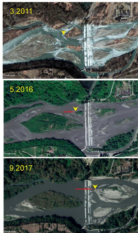
**Figure 11.** Bars and islands passing the barrage of the Malo–Kabardian irrigation system at different dates (yellow numbers). The yellow arrow shows the head of the island, passing the barrage; the red arrow shows the distance the island head moved during the period between images from Google Earth.
