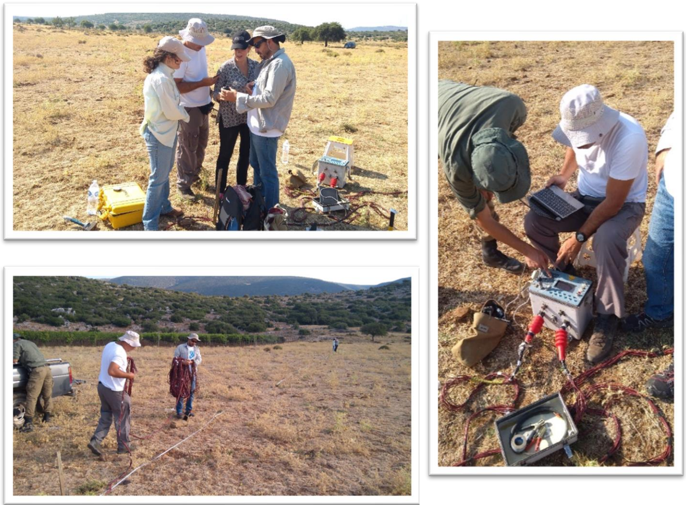
Figure 3. On the site of Meteles plain arranging ERT measurements (© IL). Upper left: four of the co-authors preparing for the ERT measurements in situ, Left: two co-authors lay the cables for ERT, Right: taking a reading in situ.
